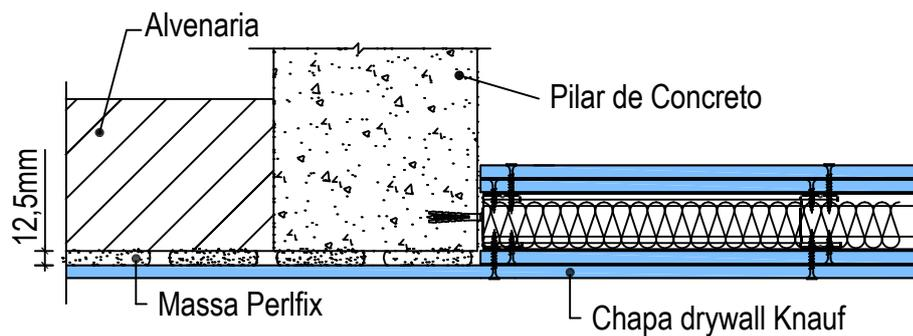
**1** **DETALHE PAREDE DRYWALL E REVESTIMENTO**
